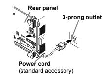
Rated supply voltage: 100 to 120VAC or 220 to 240 VAC Rated supply voltage frequency: 50/60 Hz Allowable supply voltage range: 90 to 132 VAC or 198 to 264 VAC Allowable power supply frequency range: 48 to 63 Hz
