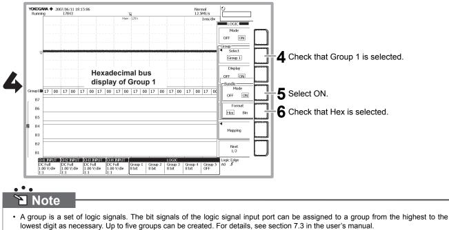
• A state display function is available. This function acquires the status of a logic signal on the point of polarity change (edge) of a specified clock signal. The state is held until the next clock occurs even if the input logic signal changes. For details, see section 7.3 in the user's manual.
