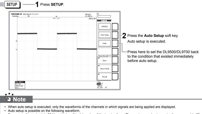
Frequency: Approximately 50 Hz or higher. Absolute value of the input voltage: The maximum value is greater than or equal to 20 mV (1:1). Type: Repetitive waveform (not complicated).
