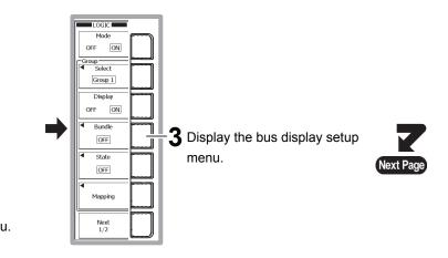
We will change the logic signal of Group 1 from bit display to hexadecimal bus display.
