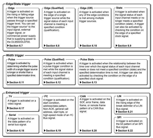
\* Trigger source refers to the signal that is used in checking the trigger condition.
